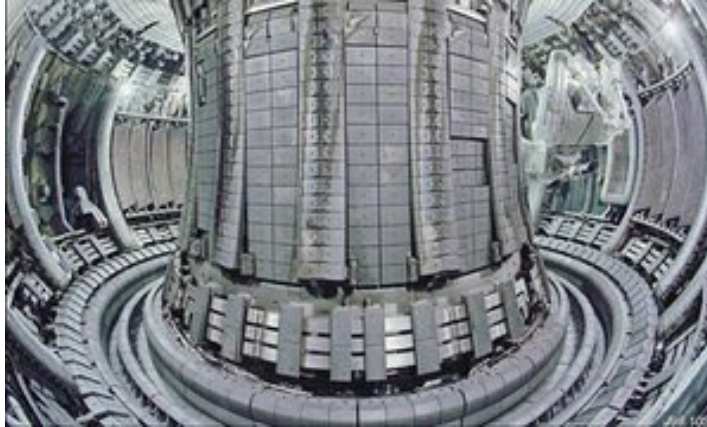
The toroidal magnetic chamber (Tokamak) of the Joint European Torus (JET) at the Culham Science Centre. Photograph: AFP/Getty Images
